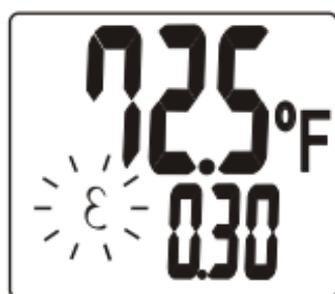
Press and hold the trigger , then press **MODE** button , flash ε displays on the screen . Please refer to the emissivity table on pages 12,13 and 14 ,emissivity value is adjustable from 0.30 to 1.0.
