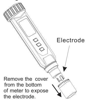
2. Dip the electrode into the test solution. Press "  $\Phi$  " to power on the meter and tir it to get a stable reading.
